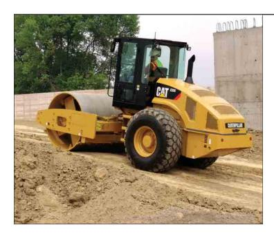
**Propel pump system.** The dual propel pump system has dedicated pumps to independently drive the heavy-duty, high-torque rear wheel and drum motors. Should loss of traction to either motor occur, there is always hydraulic flow to the non-spinning motor, allowing continuous tractive effort.
