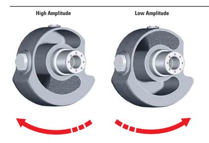
**Amplitude selection.** Positive amplitude selection is accomplished when the steel shot is repositioned inside the hollow eccentric weight. Direction of weight shaft rotation determines amplitude level.
