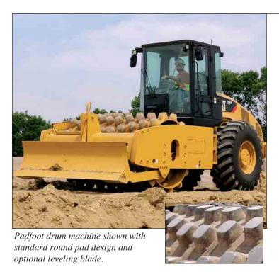
**Padfoot drum.** The padfoot drum has 140 pads welded on the drum in a chevron arrangement.
