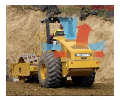
**Optimized air flow.** Pulls cool air from the middle of the hood and discharges hot air out the rear.
