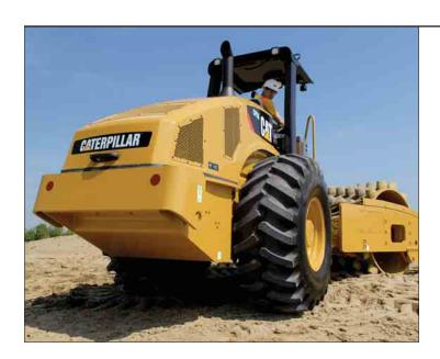
**Visibility.** The line of sight to the tire edges and rear of machine is exceptional. Operator can see obstacles measuring 1 meter high located 1 meter to the rear of the machine. Fenders have been narrowed, as has the rear bumper. Excellent visibility increases productivity when working near obstructions or maneuvering around the job site.
