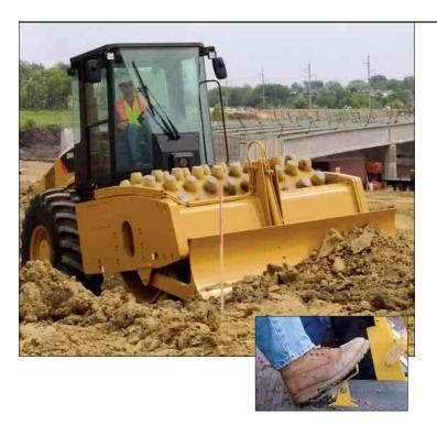
**Machine versatility and utilization.** Suitable for many applications like material knockdown, site leveling, trench backfilling and light dozing.
